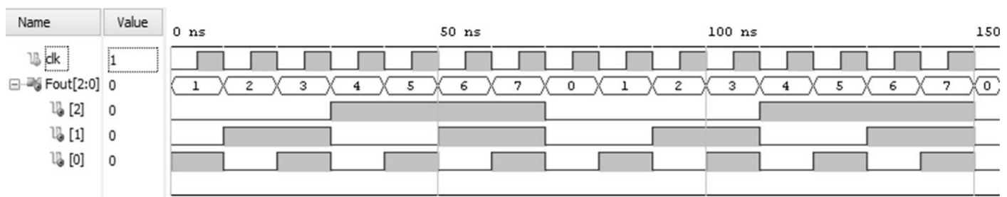
FIGURE 10.15 Frequency division results of synchronous frequency divider.
